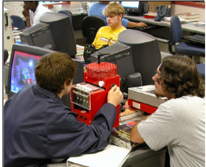
Other modules make use of special trainers that incorporate actual vehicle components, such as this DIS (Distributorless Ignition System) trainer.
